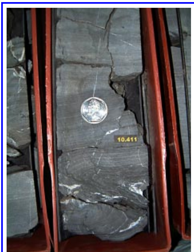
Figure 4. Drag folds along one of the thrust faults encountered in a Lake Maracaibo core which was drilled at the crest of the structure of the extracted seismic line from the 3D volume shown in Fig. 3.
